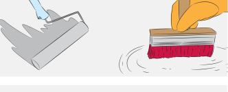
Priming the surface will also enhance the water resistance of the tiling installation, such as showers and balconies, particularly when used in conjunction with adhesive and grout where TAL Bond Powder has been added to the mix. Tip: for a fully waterproofed installation the correct waterproofing system needs to be applied before tiling.
